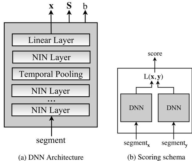
**Fig. 2.** Diagram of the DNN and scoring method.
