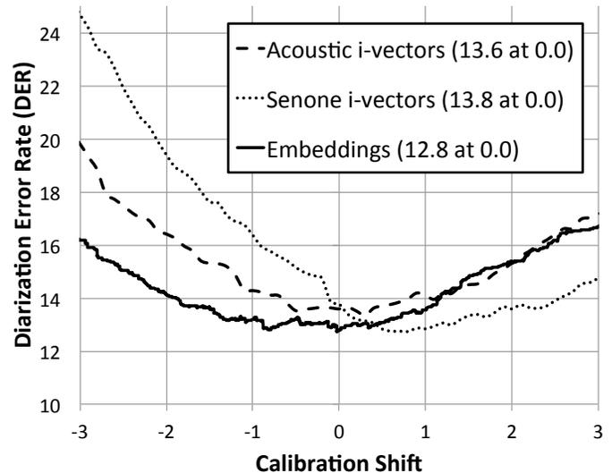
**Fig. 3.** A comparison of DER for the two baselines and the proposed embeddings for a range of calibration shifts. A geometrically decaying prior is used for number of speakers for all three systems, and, as a result, the optimal performance range is widened and centered.
