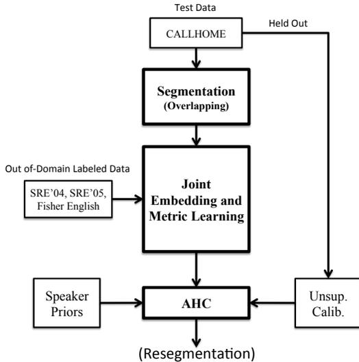
**Fig. 1.** System diagram for the diarization system presented here. This architecture is simpler than that in [5], with the i-vector extraction and PLDA steps merging into the joint embedding and metric learning, and with UBM and T entirely removed.
